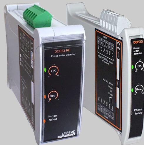
The DOP23 relay is for monitoring phase order on a three phase electrical system that can be changed and whose direction of rotation is important (eg. Pumps, saws and drills). An output contact indicating the correct sequence order of the phase and the presence of all phases can be used to validate the power on of the installation. The LEDs on the front panel allow easy diagnosis (normal, reverse order or phase failure).
